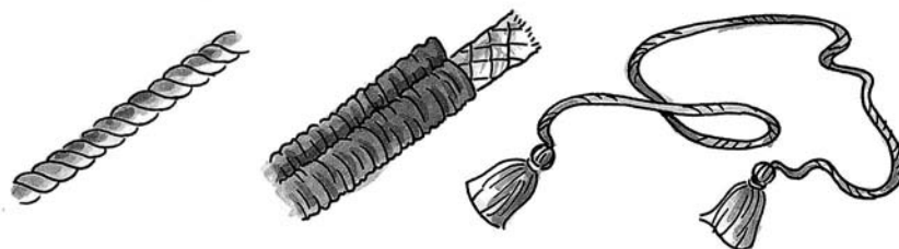
Figure 12-2: Cable cord, filler cord, and chair tie.
