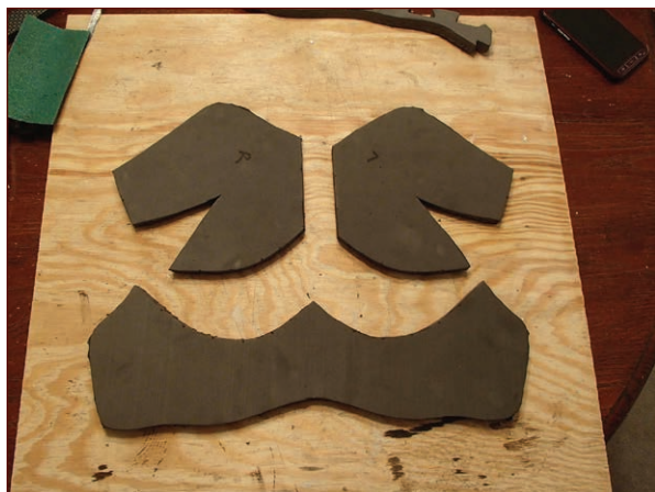
FIGURE 3-48: Cutting out the foam parts based on the paper templates
