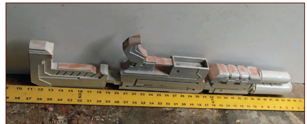
FIGURE 1-86: Gluing the pieces together, with a straight edge in place for alignment
