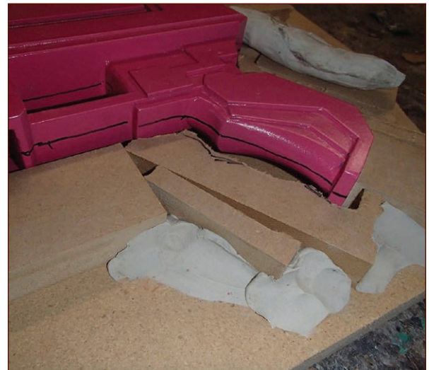
FIGURE 7-22: Blobs of clay to stick the blocks of scrap to the work surface
