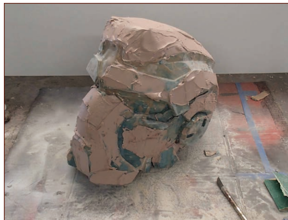
FIGURE 2-47: The first coat of Bondo
