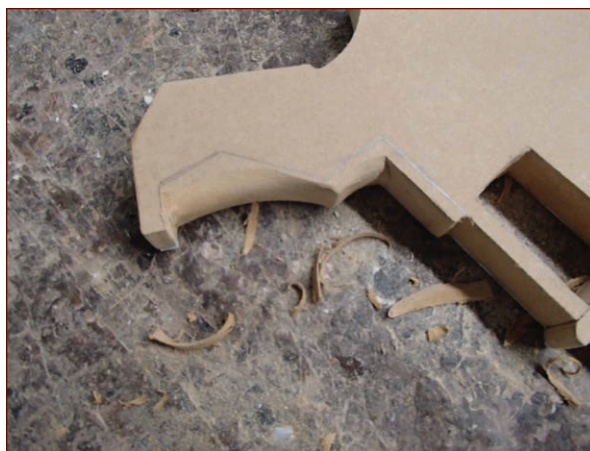
FIGURE 1-63: The front of the grip after whittling it round with a utility knife
