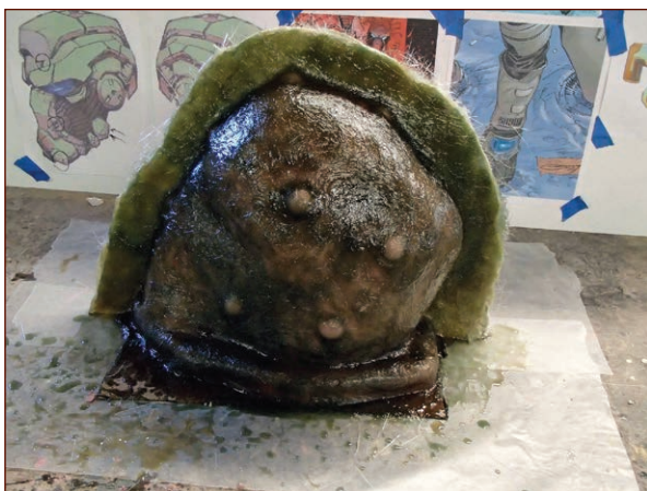
FIGURE 8-21: Fiberglass laid up across the rest of the mold
