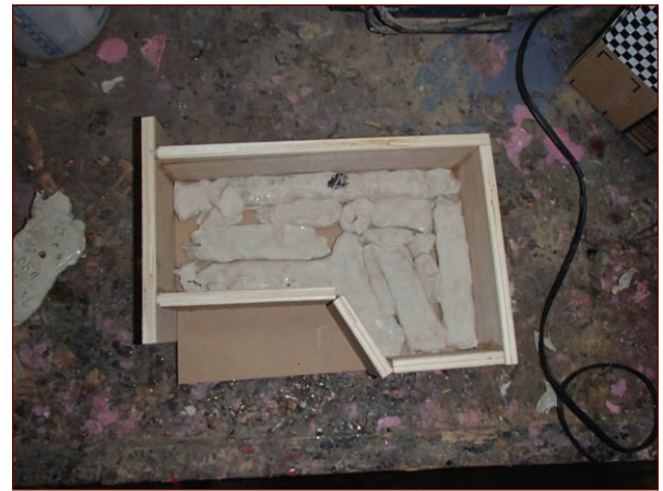
FIGURE 7-4: The clay bed built up for the prototype to rest on.
