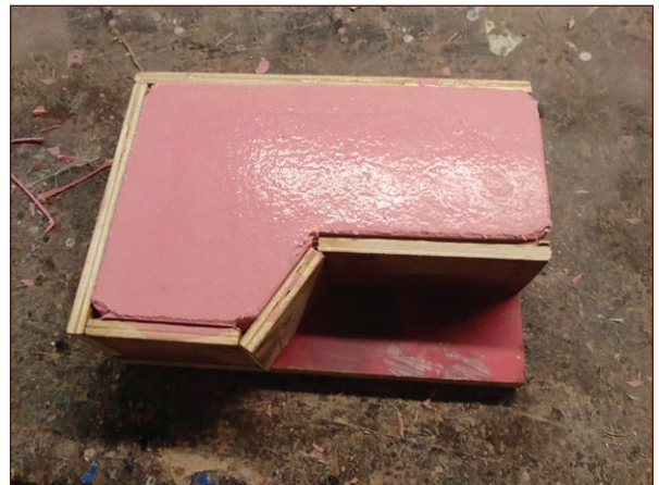
FIGURE 7-14: The reassembled mold box, without top
