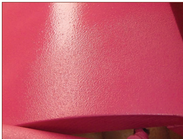
FIGURE 11-12: This surface might be okay for citrus fruits, but not for a glossy coat of paint
