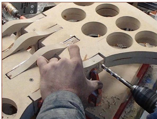
FIGURE 1-27: Making a bigger hole for the screw head to hide in is called "countersinking."
