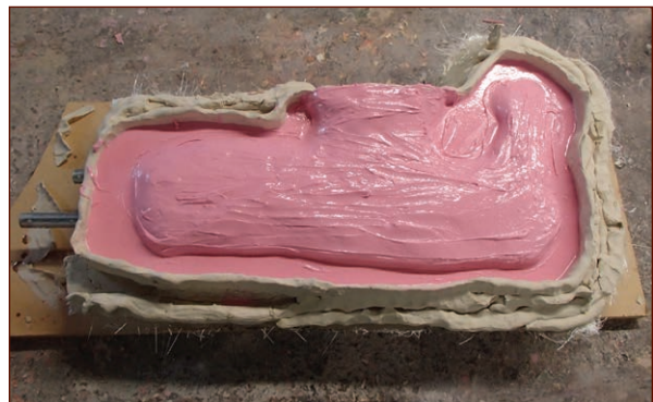
FIGURE 7-43: The thickened rubber jacket
