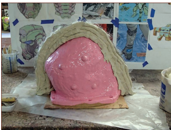
FIGURE 8-22: By the time you're looking at this angle, you're halfway done with the mother mold.
