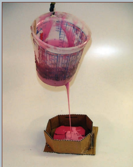
FIGURE 6-7: An inexpensive de-gassing plan
