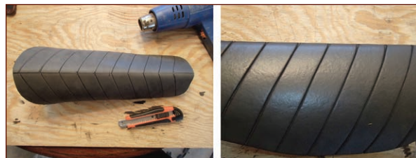
FIGURE 3-52: Making a seam line that's only skin deep
