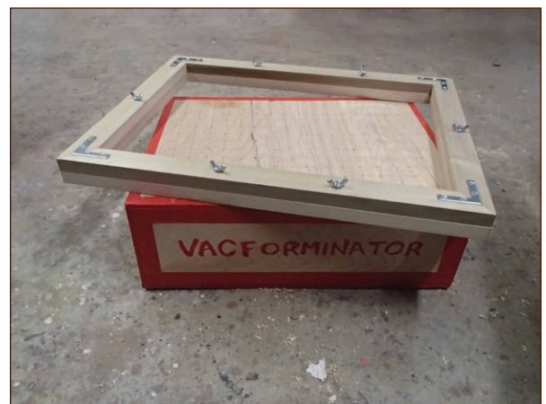
FIGURE 9-28: With the edges taped and a name added to the box, the vacforming apparatus is complete.
