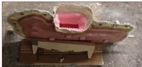
FIGURE 7-52: The mold wedged into position for the last section to be made
