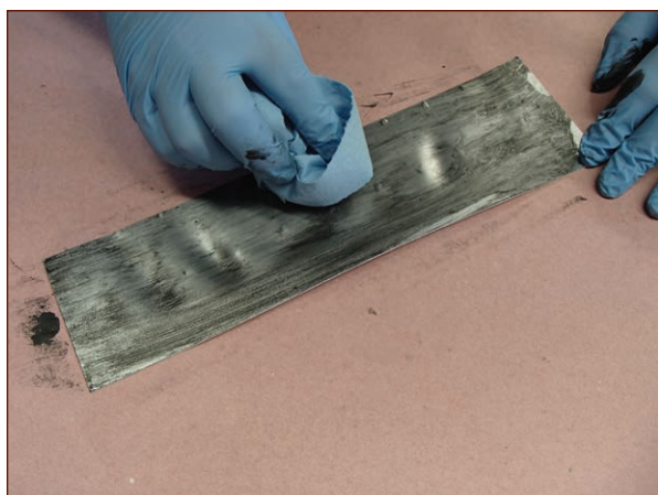
FIGURE 12-6: Gently removing most, but not all, of the black paint with a rag leaves streaks behind.
