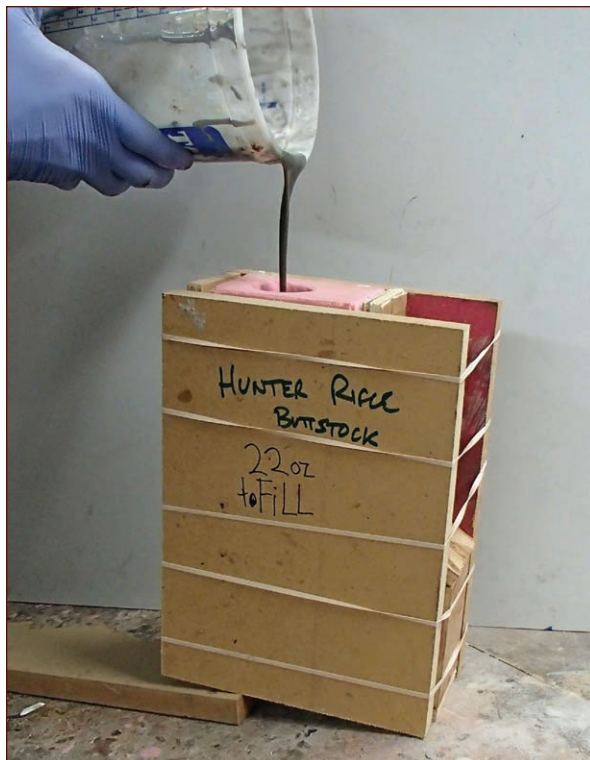
FIGURE 7-16: Pouring in some resin
