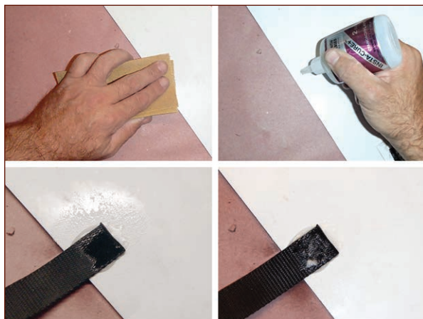
FIGURE 14-10: Gluing nylon straps to a styrene sheet with CA adhesive
