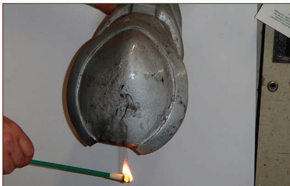
FIGURE 13-49: Sooty smoke sticking to the wet clearcoat
