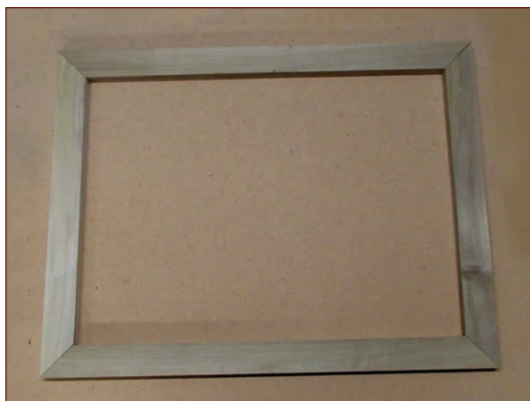
FIGURE 9-19: Wooden parts for one side of the vacforming frame
