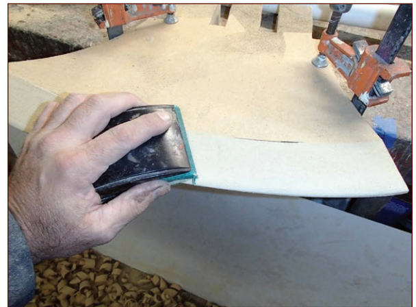
FIGURE 1-19: Fine-tuning the blade shape with a sanding block
