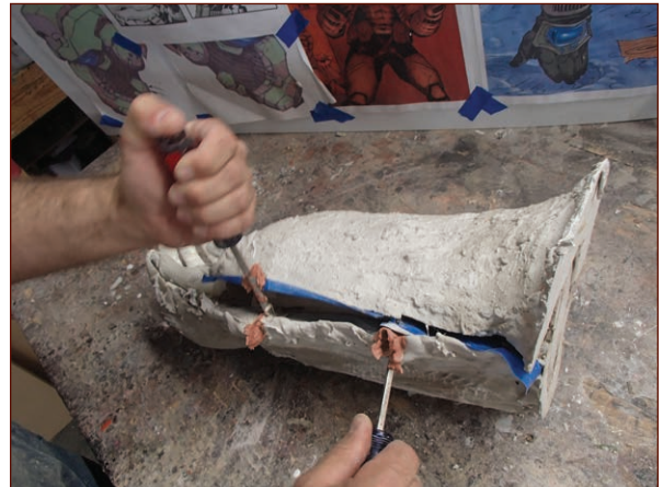
FIGURE 9-13: Using a pair of screwdrivers to gently pry apart the two halves of the plaster mold
