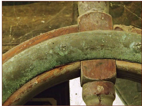
FIGURE 13-42: A strip of bronze after years in a marine environment
