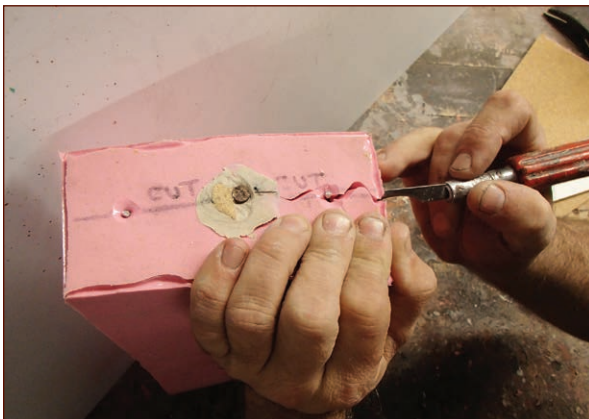
FIGURE 6-31: An initial serpentine cut in the top of the mold
