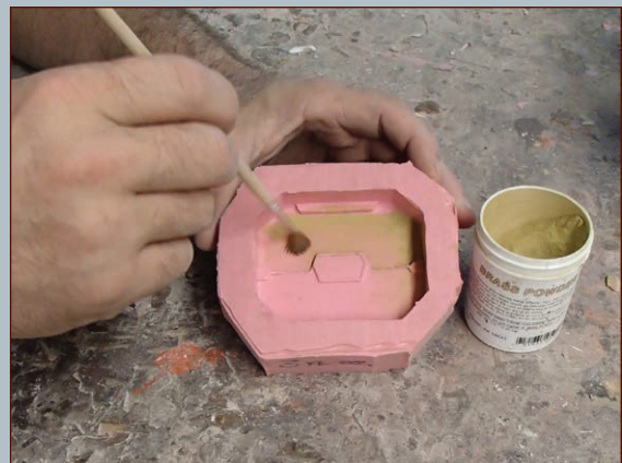
FIGURE 6-17: Dusting the mold with powdered brass
