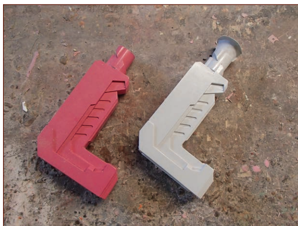
FIGURE 7-17: The first cast part pulled out of the mold
