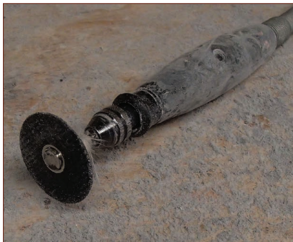
FIGURE 8-34: The cut-off wheel
