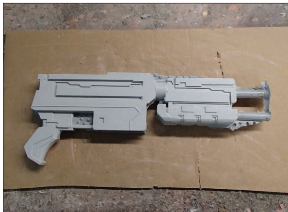
FIGURE 7-61: Fresh, hot, cast part removed from the mold
