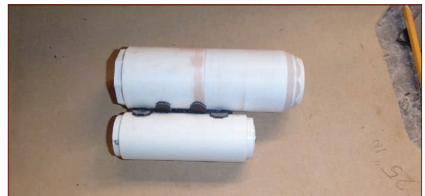
FIGURE 1-78: The finished barrel assembly, ready for primer
