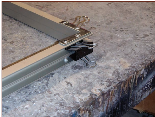
FIGURE 10-8: Binder clips make a pair of rectangles into an actual clamping frame.
