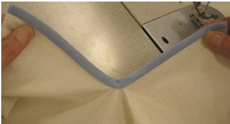
Figure 9 Bound slit opening.
