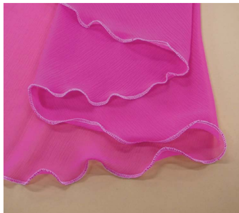
Figure 48 Rolled edge hem using 504 Three Thread Overedge.
