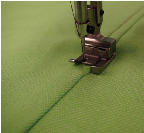
Figure 17 Topstitching using Lockstitch (301).
