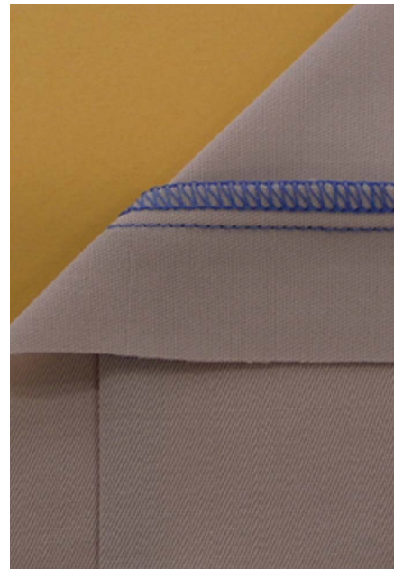
Figure 39 516 Five Thread Overedge.
