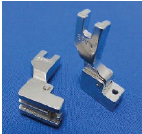
Figure 7 When inserting an invisible zip, the presser foot shown is used to enable the stitching to be located close to the teeth of the zip. The zip is attached to the garment before the seam is joined and it is attached with the zip itself fully open.
