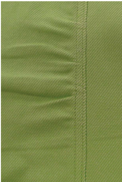
Figure 2 A seam with poor appearance; it has ripples known as seam pucker along the seam length.
