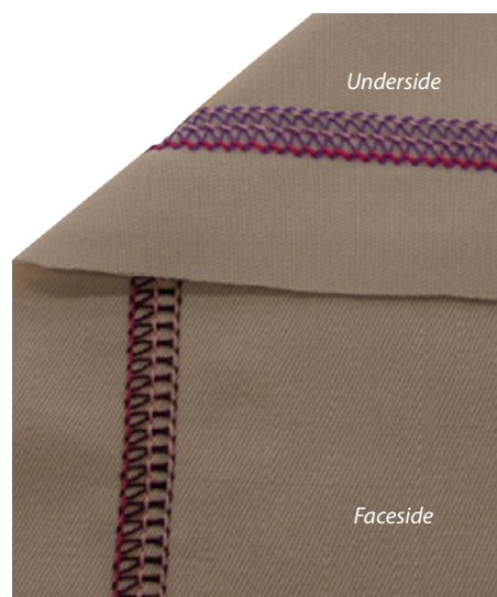
Figure 29 Three Needle Cover Chainstitch (605).
