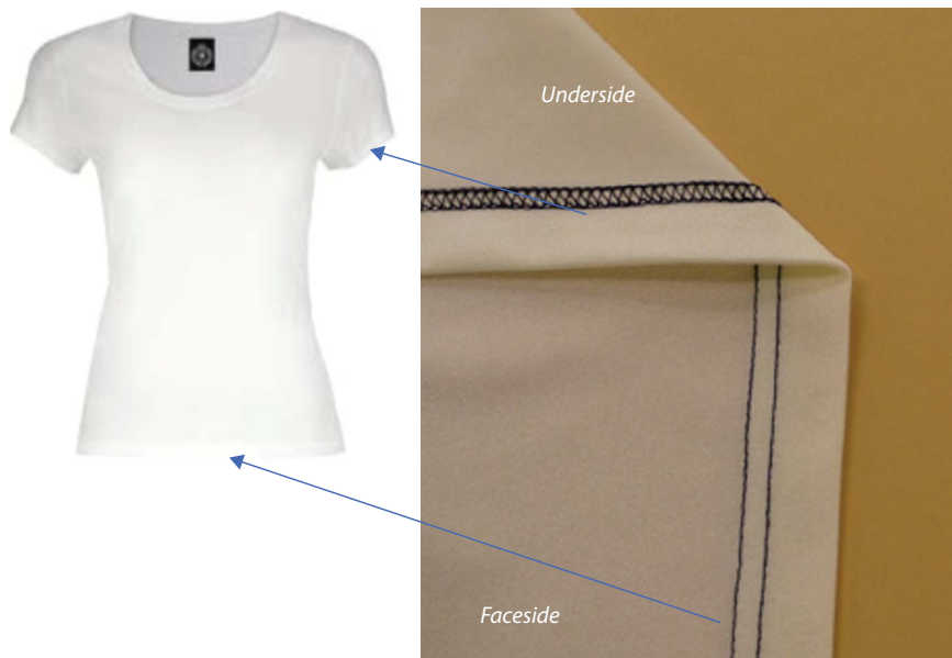
Figure 26 Two Needle Chainstitch Bottom Cover (406) used for hemming.
