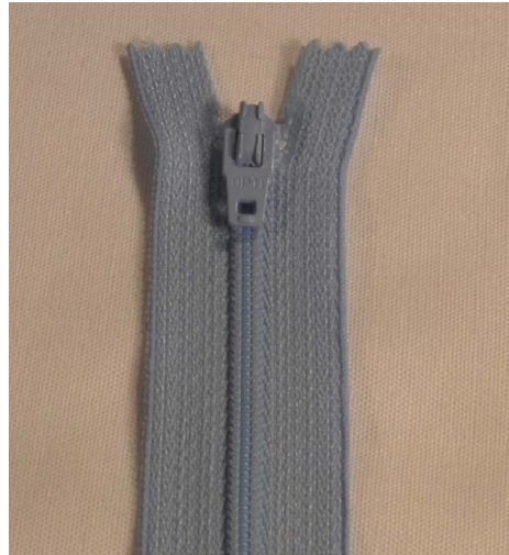
Figure 2 The teeth can be made from a continuous coil of polyester monofilament with a slider that, when moved, links or unlinks the teeth.
