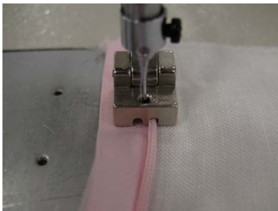
Figure 12 Invisible Presser Foot.
