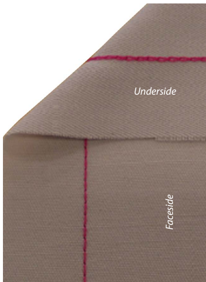
Figure 20 Single Thread Chainstitch (101).
