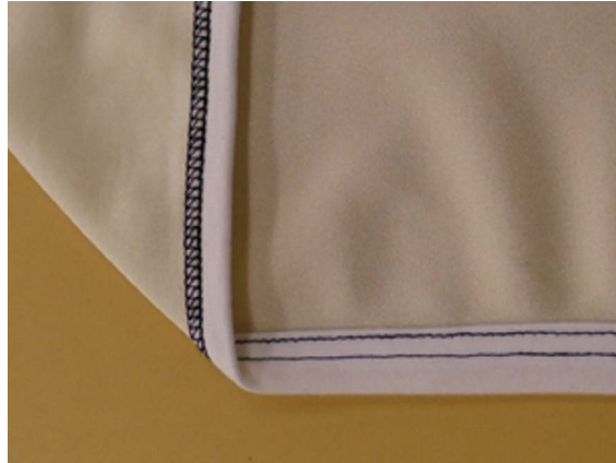
Figure 27 Two Needle Chainstitch Bottom Cover (406) used for attaching binding.
