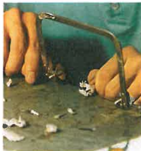
Photo 1: Removing the eagle's head using a fret saw with a fine blade
