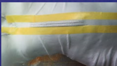
Zip area masked off prior to applying putty
