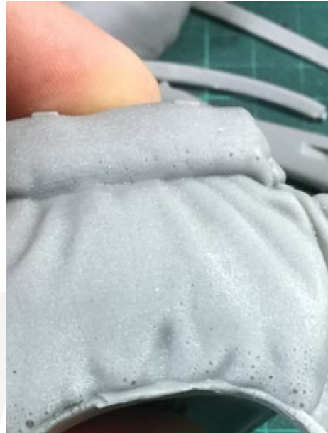
Sub-surface air bubbles
