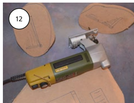
12. I cut the base with my jigsaw and used sandpaper to sand down the edges.
