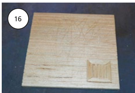
16. The rooftop was done by engraving a planked floor onto the 10,5 x 10,5 cm balsa wood. The wooden hatch was done from 1,5mm balsa wood.
