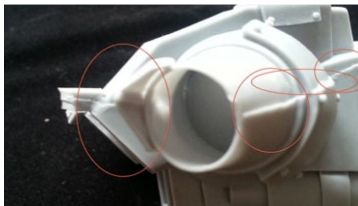
Detailed flash lines and blocks on the back of the exhaust of the body.
