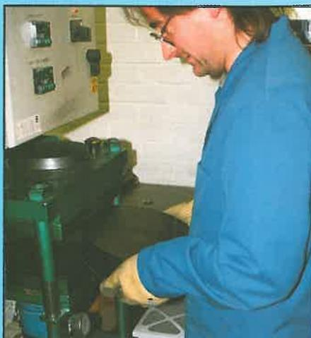
*Placing the master mould in the press.*
