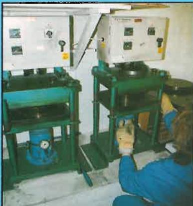
*A master mould is pressed into shape.*
