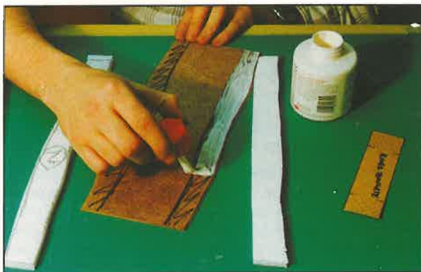
Gluing the banks to the baseboard.
