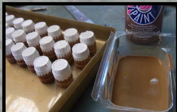
Figure 4: dipping pieces in watered-down cheap hobby paint or even house paint gives an excellent cover over plaster pieces.
