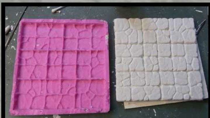
Figure 1: a mold was made of a floor section.
